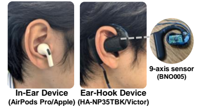
Fig. 6. In-ear devices and ear-hook devices. Location of the 9-axis sensor.
